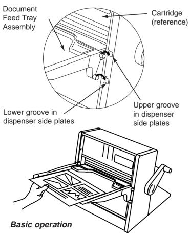
Step 1 - Insert and align document on feed tray. Extend the document completely into the cartridge opening. Align to the left for letter size documents, to the right for A3/A4 documents.
